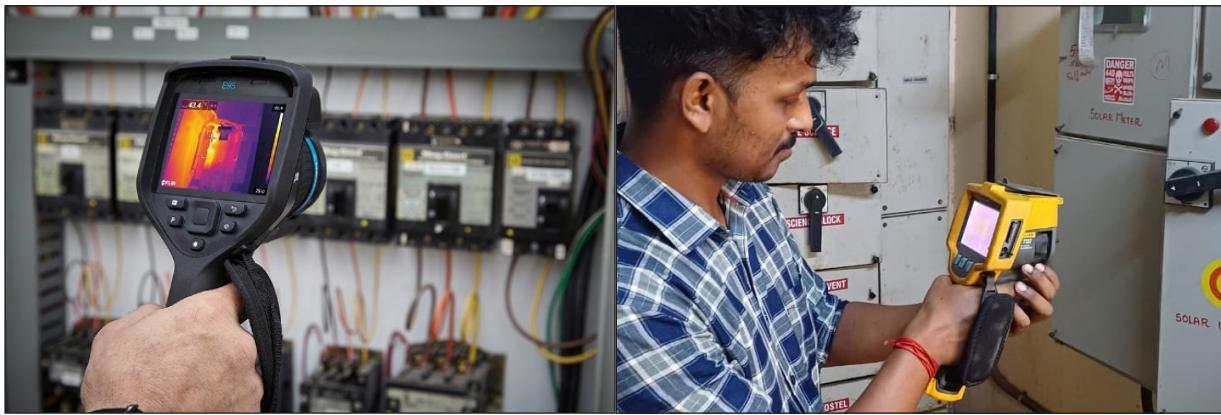
Fig 4.21. Thermal imaging
