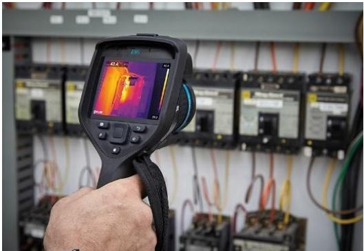
Fig. 4.35 Taking thermal imaging data
