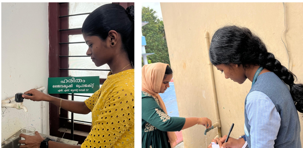
Fig 5.7 Field-Based Manual Water Discharge Collection- Zone two
