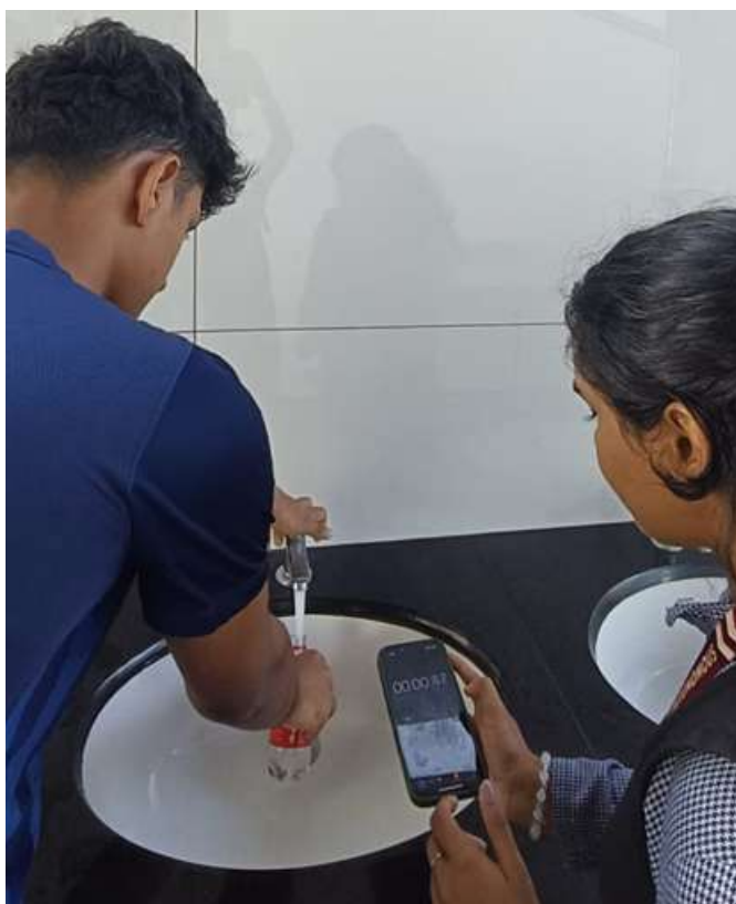
Fig 5.6 Manual water discharge sampling
