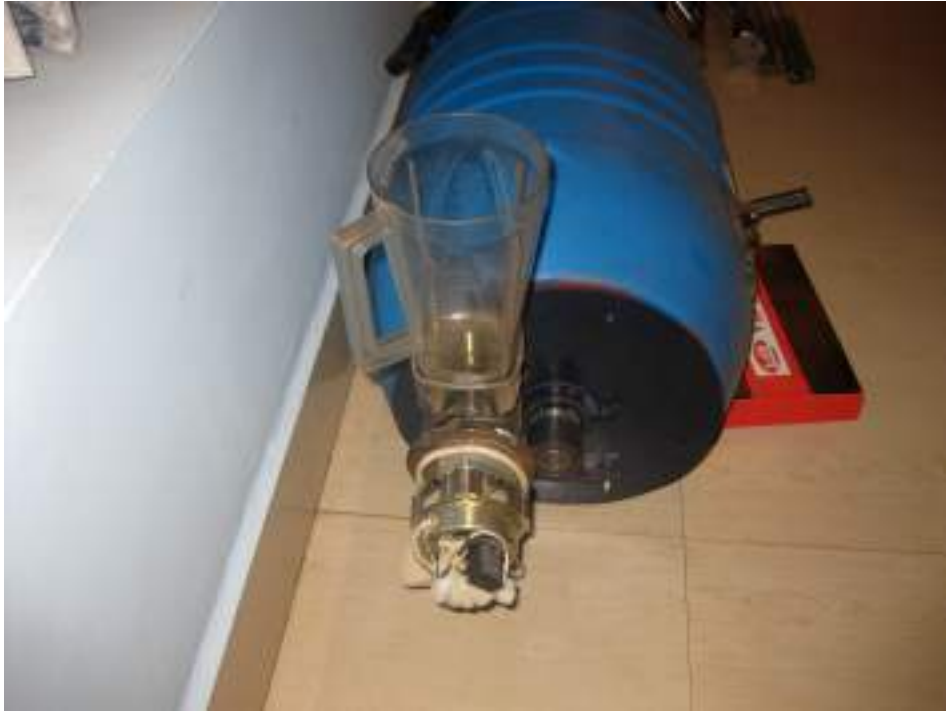
Fig. 15. Grinder fitted at the mouth of the barrel for grinding into short pieces of the waste materials.
