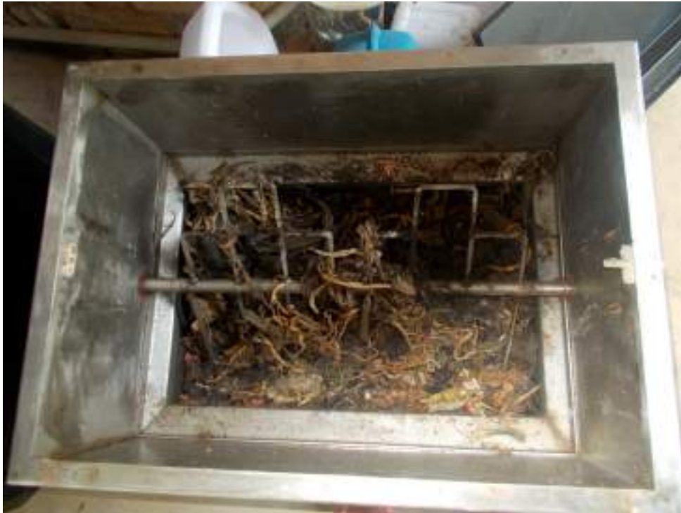
Fig. 10. Decomposing kitchen waste inside the upper chamber of the machine
