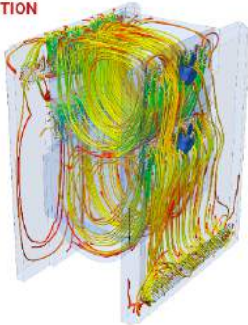
Fig. 12. Computer simulation of air flow inside the machine
