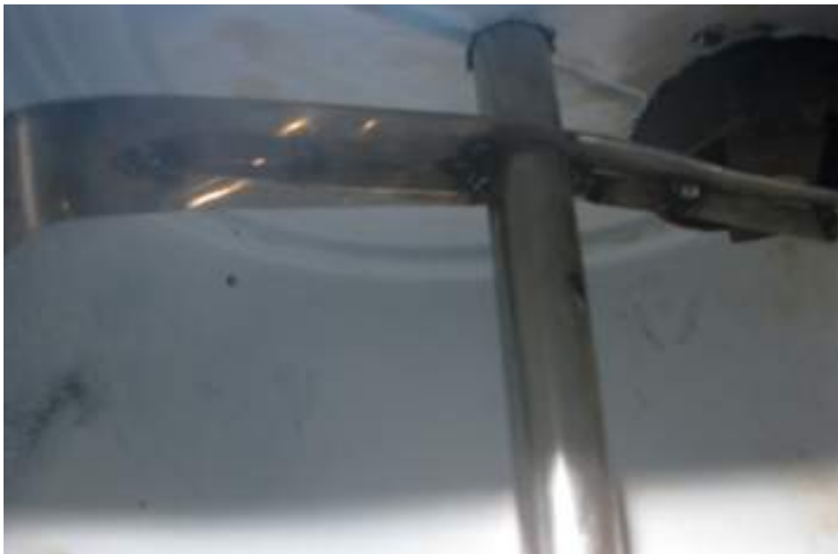
Fig. 15. Grinder fitted at the mouth of the barrel for grinding into short pieces of the waste materials.
