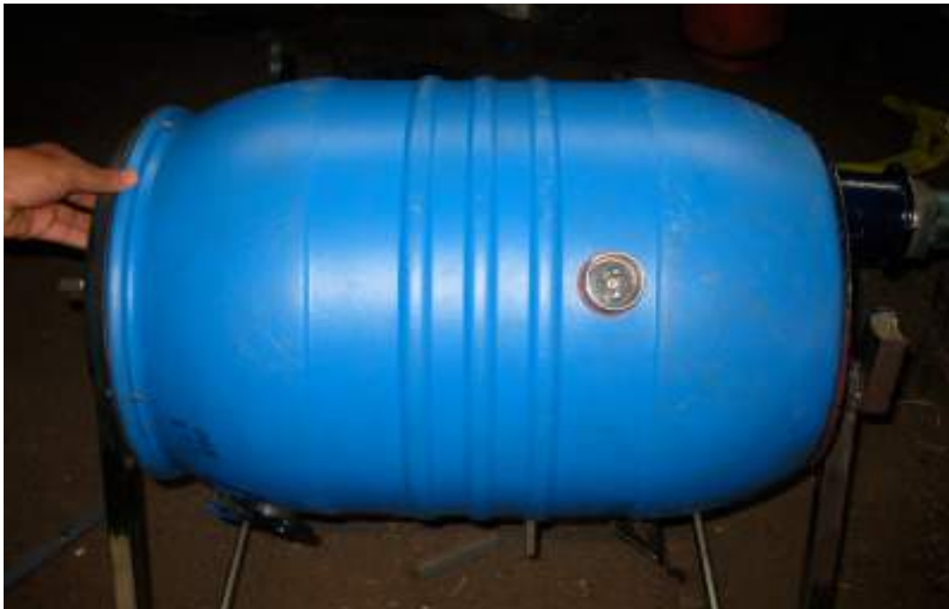
Fig. 14. Plastic barrel fixed with a heating element for intermittent heating for promoting thermophilic microbial inoculum.
