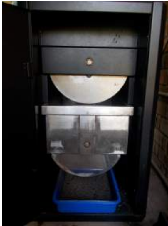
Fig. 8. Interior of the composting machine with 3 chambers. Compost collected at bottom tray.
