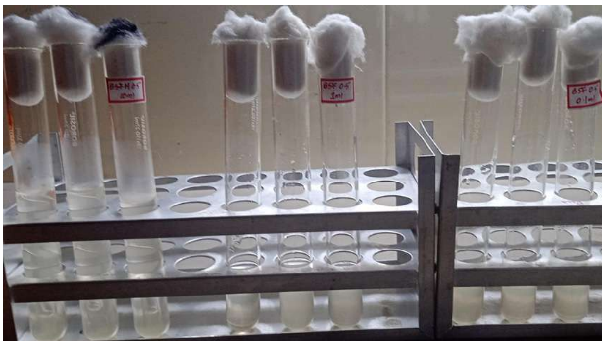
Figure 21. Fecal coliform analysis of samples
