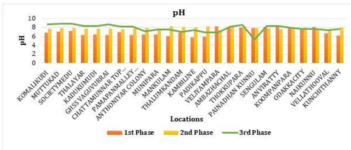
Graph 3. Phase-wise comparison of pH levels in water samples collected from biosand filters across various locations.
