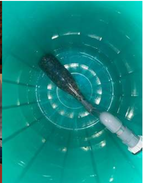
Figure 11. Water bottle placed in the bottom of the filter
