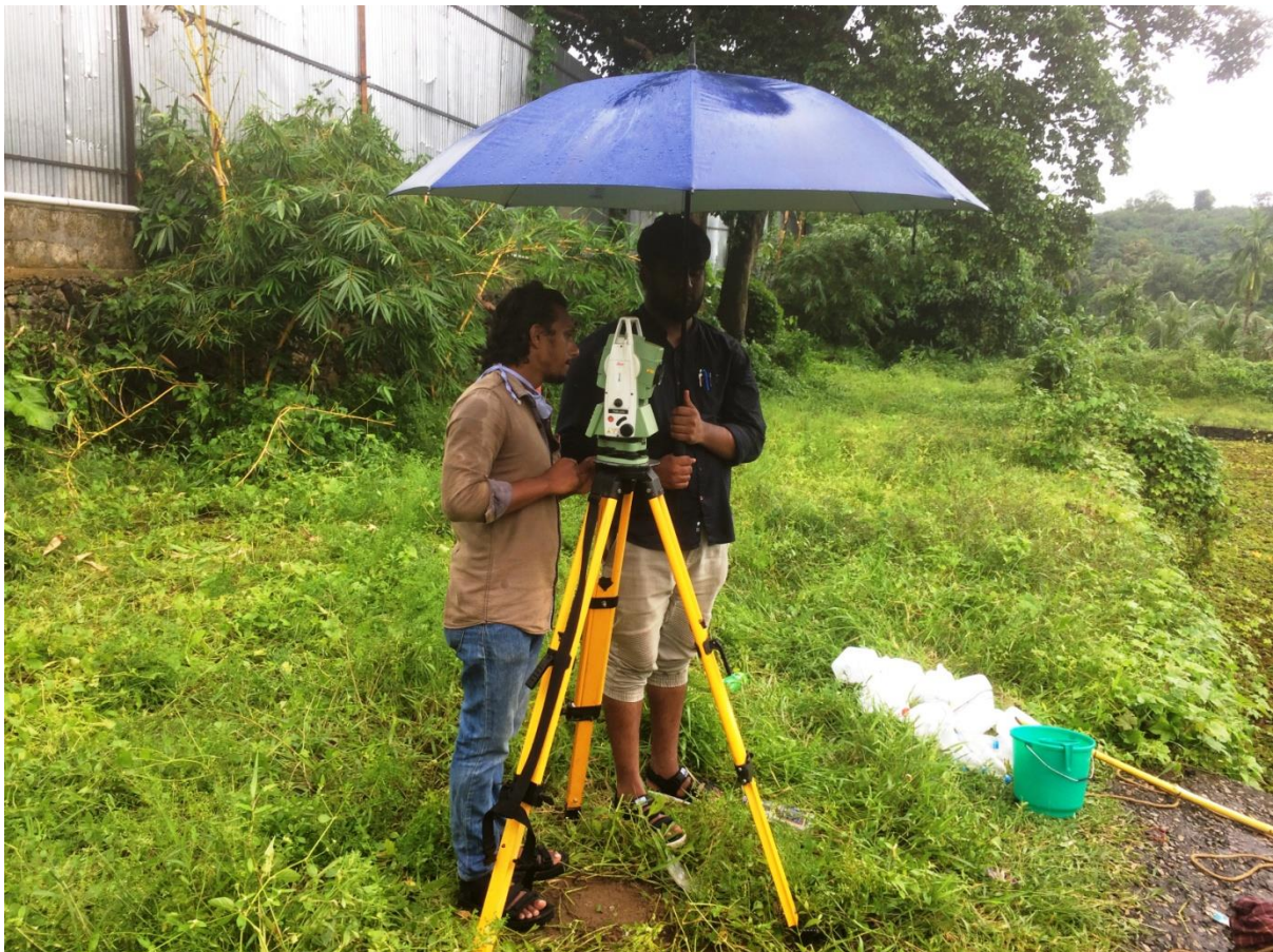
Fig. 2.2. Survey of the pond area using Total station
